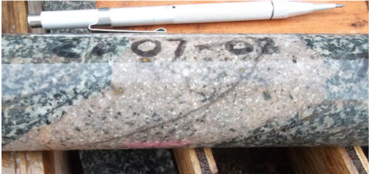
Figure 3 - Hornblende feldspar porphyry dike intersected in 2007 diamond drilling at Trident. The key question remains — where is the rest of the system?
