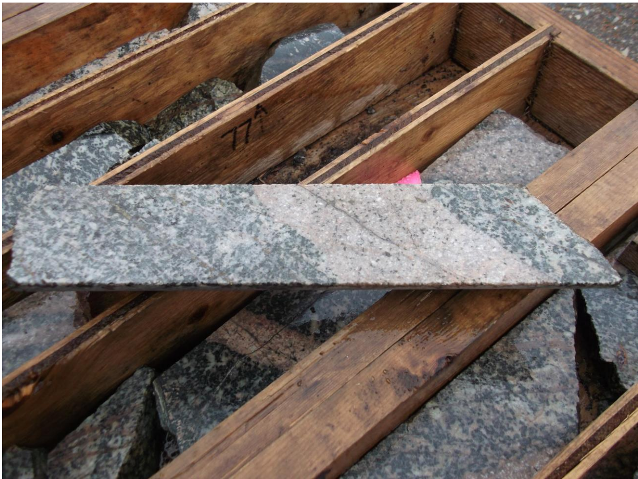
Figure 1 - Example of mineralized porphyry dikes within a 6 m interval grading 0.87% copper (2007-2 from 74 - 80m)
