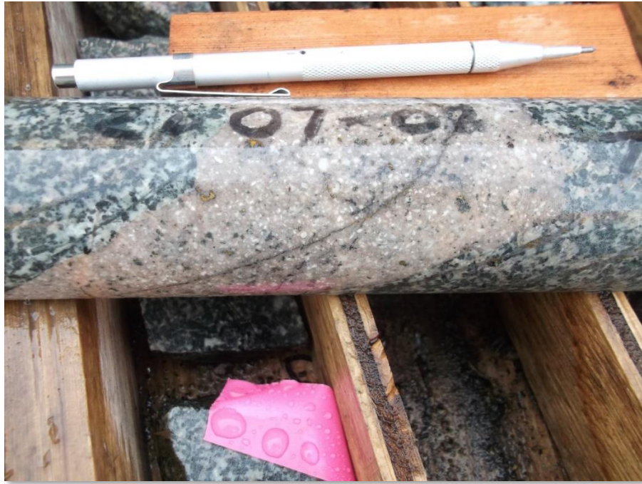
Porphyry intrusion in DDH-2007-2 @ 77m with chalcopyrite as blebs, disseminations and veinlets (note emplacement of sheeted quartz veins appears to precede emplacement of porphyry)
