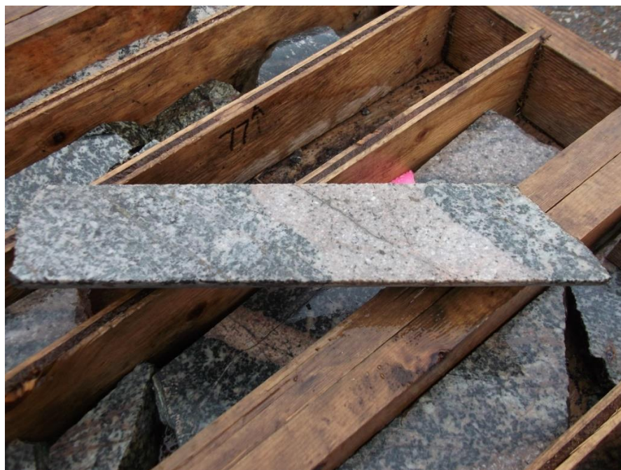
Porphyry intrusion and mineralization in DDH-2007-2 @ 77m associated with sheeted quartz-sulphide veining
