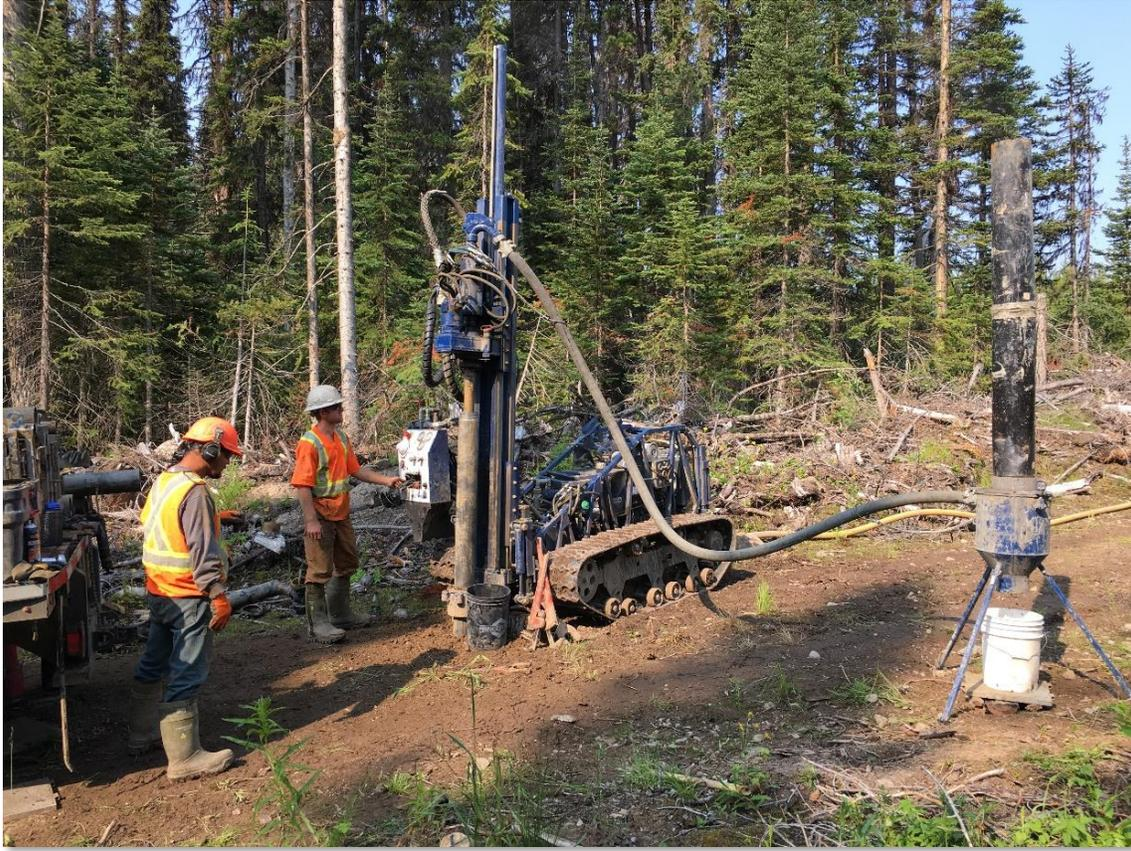
*Figure 2 - 2019 Reverse Circulation Drill at the Bulkley Project*
