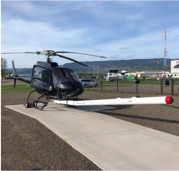
"Stinger" magnetometer mounted to helicopter
