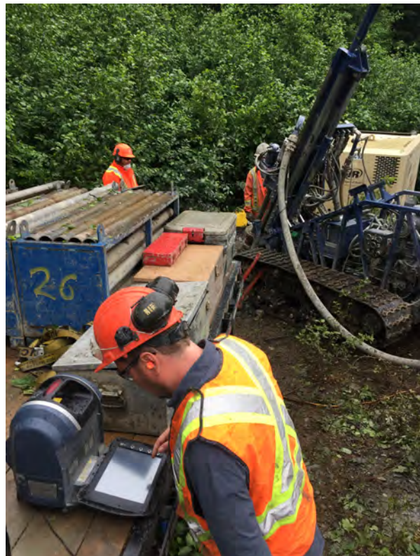
PEMC's portable XRF analyzer and RC drill at the Kitimat Property.
