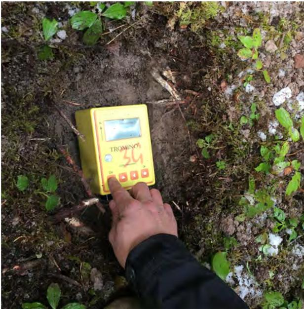
*Passive seismometer collecting subsurface data*
