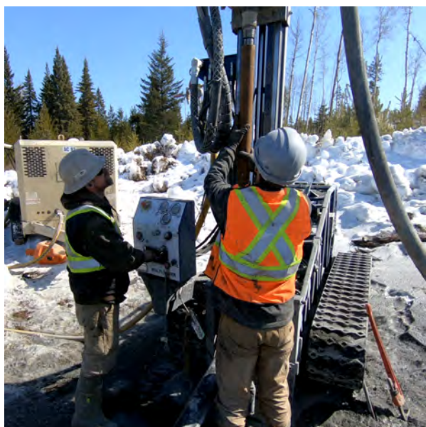
2018 Reverse Circulation Drilling at the Red Property
