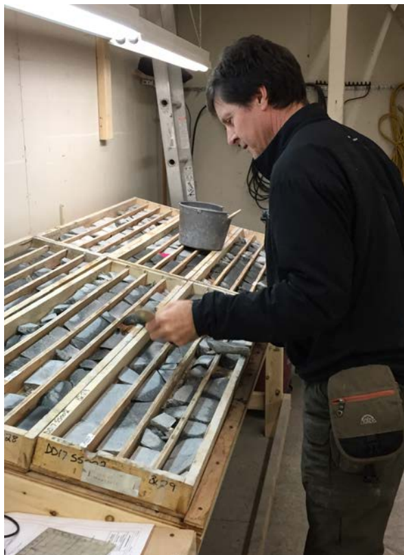
PEMC advisor Dr. Paul Johnston inspecting diamond drill core from 2018 partner funded drilling at the Stars Project.
