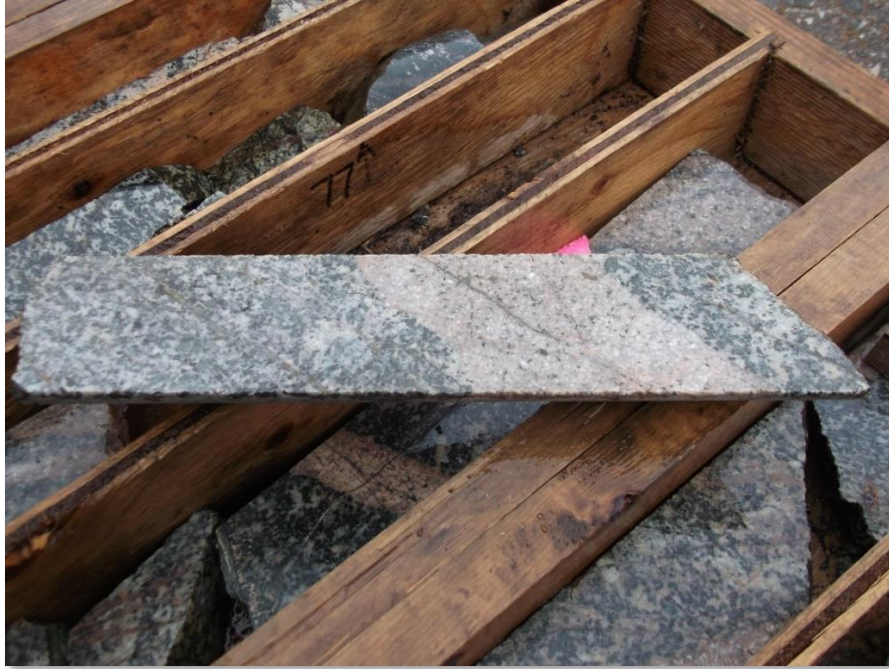
Porphyry intrusion and copper-gold mineralization in DDH-2007-2 @ 77m associated with sheeted quartz-sulphide veining
