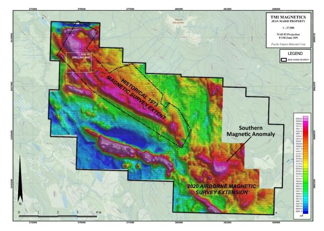
Figure 4 - 2020 Airborne Magnetic Survey (TMI)
