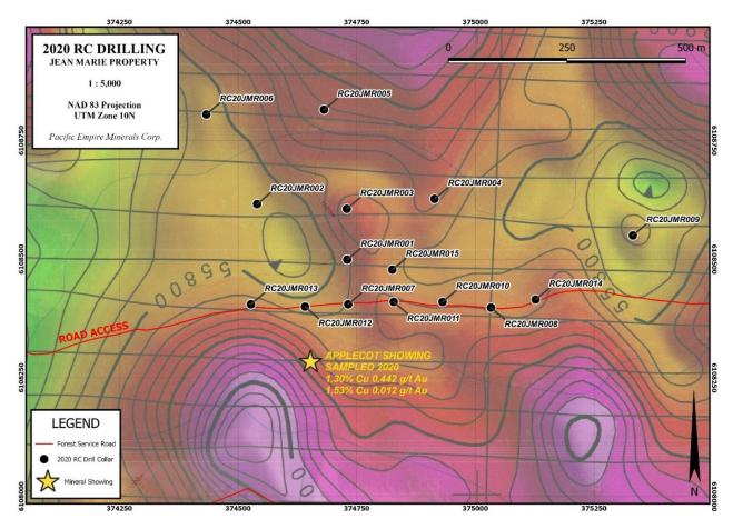
Figure 1 - 2020 RC Collar Locations with 2020 Airborne Magnetics (TMI)
