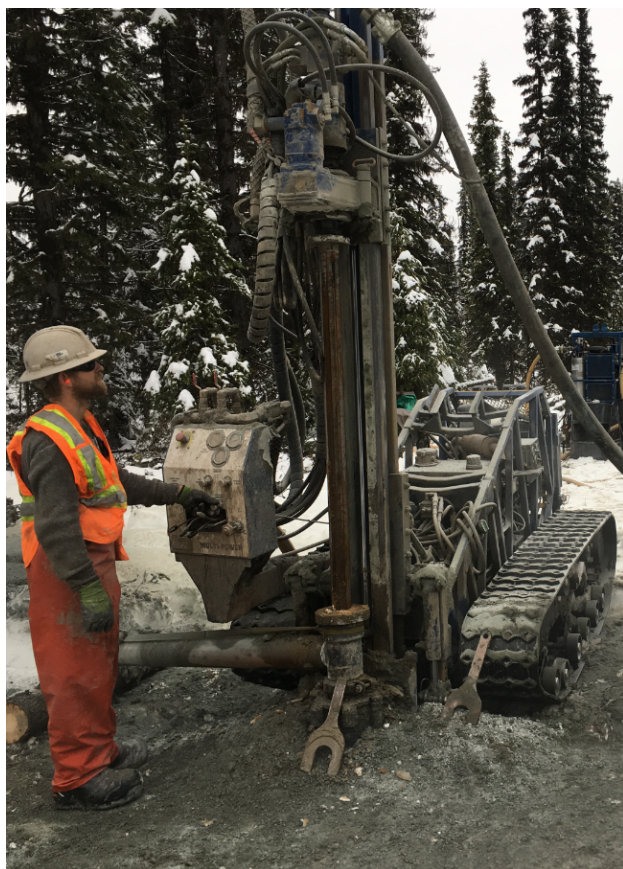
Ongoing RC Drilling at Elbow Zone
