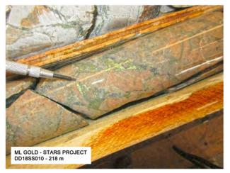
Potassically altered feldspar porphyry with chalcopyrite -Sampled 12.2 m @ 0.48% Cu from hole DD18SS010
