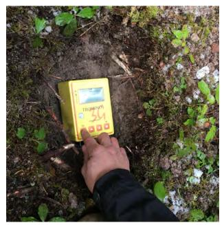
Passive seismometer collecting subsurface data
